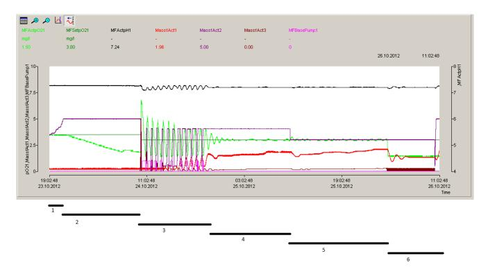
**Phase 1:** Air controller alone. The pO2 stays fix at 3.5 mg/L and the air flow rate increases.
