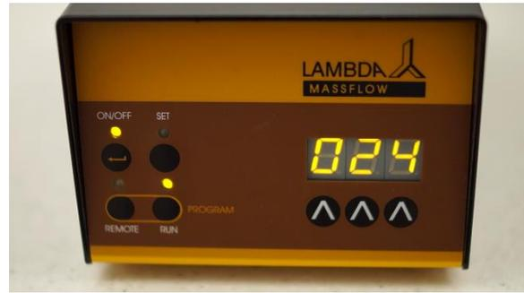
**Figure 2.1-2** Otherwise, the reading 000 (or 0.00 for MASSFLOW 5000) seen at the beginning will increase progressively until the programmed flow rate is attained. This may take about 15 seconds depending upon the selected flow rate.
