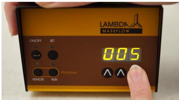
**Figure 2-5** Select the time duration of the first flow rate (for example: 005 = five minutes).
