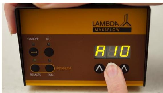
**Figure 3.4-2** Release the **SET** button. Select the desired address from 0 to 99 and press the **ON/OFF** button to save it.
