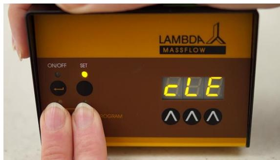
**Figure 2.3-2** Continuous pressing of **REMOTE** and **RUN** buttons even after the indication of "**PGM**" ends up with the "**cLE**" message. This indicates that the program has been deleted from the memory.
