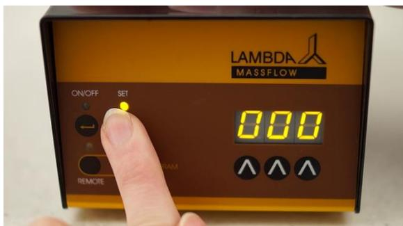
**Figure 1.3-1** Press the **SET** button. The corresponding LED will light and the display shows the pre-set value of flow rate.
