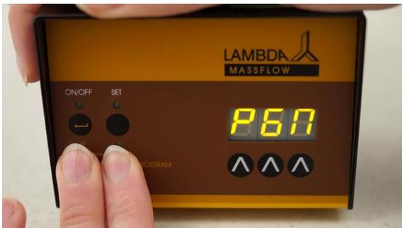
**Figure 2-1** To enter the programming sequence press simultaneously the **REMOTE** and **RUN** buttons until the message **"PGM"** appears on the display.
