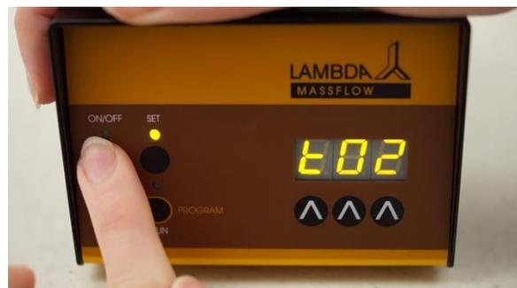
**Figure 2-8** Press the **ON/OFF** button. The message **"t02"** will shortly appear on the display followed by the duration, which has been memorized earlier.
