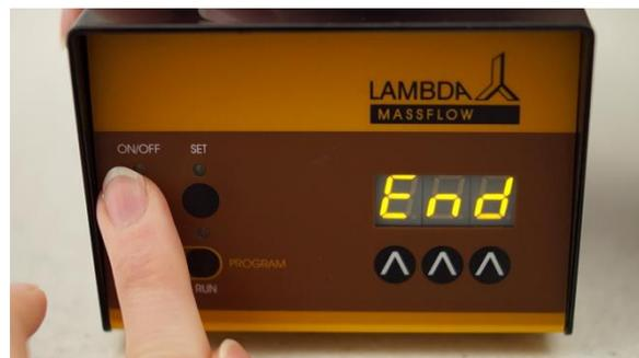
**Figure 2-14** Press the **ON/OFF** button to confirm the selected cycle. The message **"End"** will appear on the display and the instrument is ready for use.
