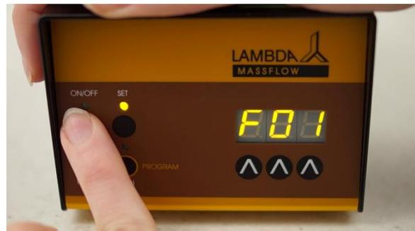
**Figure 2-2** Press the **ON/OFF** button. The message **"F01"** will appear for one second on the display followed by the value of the flow rate for the first step, which has been stored in memory.
