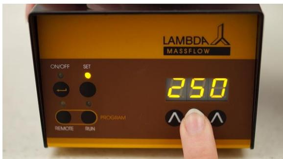
**Figure 2-7** Select the value of the flow rate of the second step by pressing the  $\wedge \wedge \wedge$  under the display.
