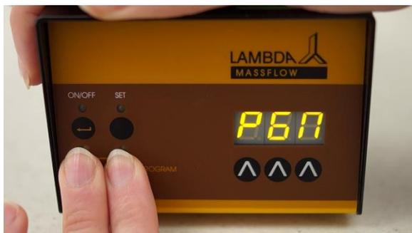
**Figure 2.3-1** Press **RUN** and **REMOTE** buttons simultaneously. The message "**PGM**" will appear on the display.
