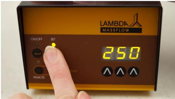
**Figure 1.3-3** Press the **SET** button again. The LED is switched off and the display shows the actual flow rate. It should indicate 0.0 l/min.
