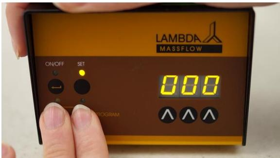
**Figure 2-11** The flow rate (000) of the next step which will not be programmed appears on the display. Do not change the flow rate (000).
