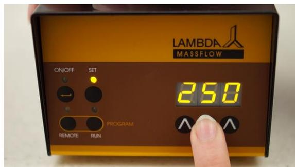
**Figure 1.3-2** Set a desired flow rate with the buttons **Λ Λ Λ** under the LED display.
