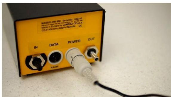
**Figure 1.1-4** Plug the connector of power supply cable into the “POWER” socket (12 V) at the rear of the MASSFLOW gas flow controller or meter and secure it.
