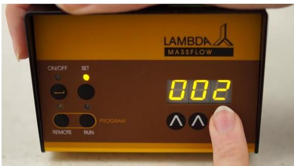
**Figure 2-13** If you wish to repeat the same program twice, increase the cycle number to **"002"** by pressing the buttons **^ ^ ^** below the display.
