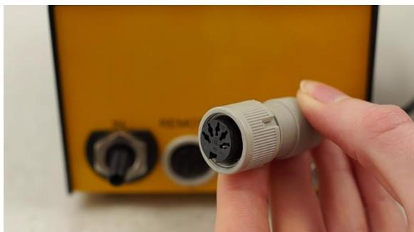
**Figure 1.1-3** 5-pole connector of the universal plug-in power supply (100-240 V AC/50-60 Hz, 12 VDC, 24 W) cable.
