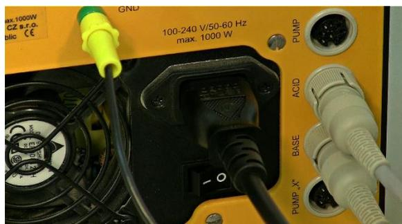
**Figure 1.1-1** One end of the 8-pole cable should be connected to the “PUMP”- socket at the rear of the MINIFOR laboratory fermenter-bioreactor control unit.
