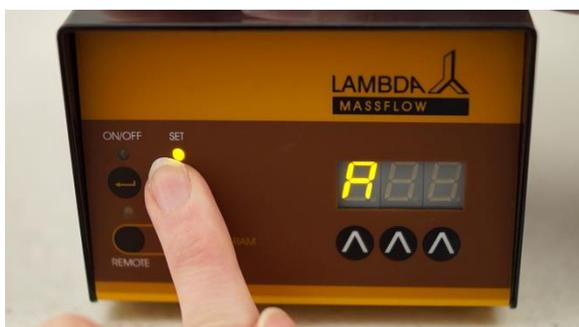
**Figure 3.4-1** Press and hold the **SET** button while plugging the cable into the socket again. The front panel illuminates and the display shows **"A00"**.
