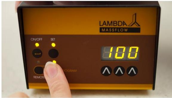
**Figure 2.1-1** The program is started by pressing the **RUN** button and the corresponding LED will light. The flow rate of the first step will appear on the display if the **SET** button is activated.
