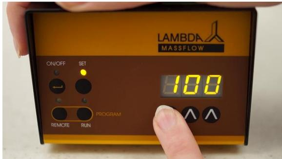
**Figure 2-3** Press the buttons  $\wedge \wedge \wedge$  under the display to select the desired flow rate value of the first step (for example: 100 ml/min for MASSFLOW 500 or 0.1 l/min for MASSFLOW 5000).
