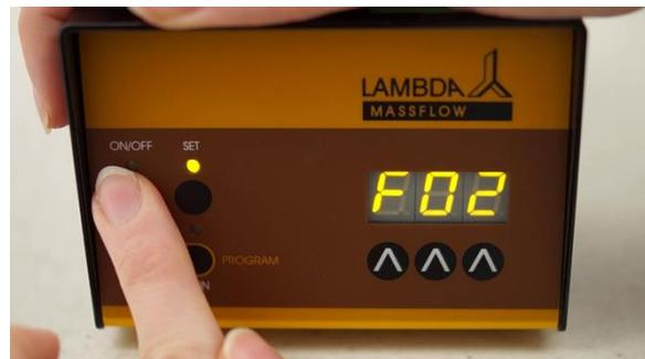
**Figure 2-6** Press the **ON/OFF** button. **"F02"** message will appear on the display and after one second, the value of the flow rate in the memory will be displayed.
