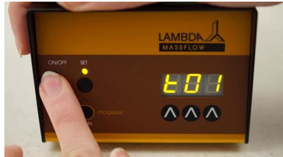
**Figure 2-4** Press the **ON/OFF** button again. The message **"t01"** will appear on the display indicating that the time period of the first step can be programmed. The display will then show the time period memorized earlier for the first step.
