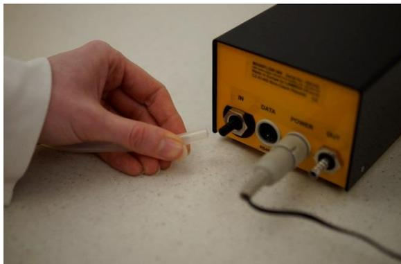
**Figure 1.2-1** Connect the gas tubing (inside diameter about 5.5 to 6 mm) to the gas **IN** nozzle and secured it in place with appropriate clamps.
