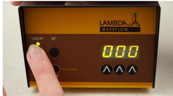
**Figure 1.3-4** Press the **ON/OFF** button. After about 10 seconds (about 30 seconds for low flow rates), the flow rate will progressively attain the pre-set value.
