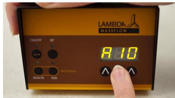
**Figure 3.4-2** Release the **SET** button. Select the desired address from 0 to 99 and press the **ON/OFF** button to save it.
