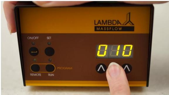
**Figure 2-9** Select the new time duration for the second flow rate.
