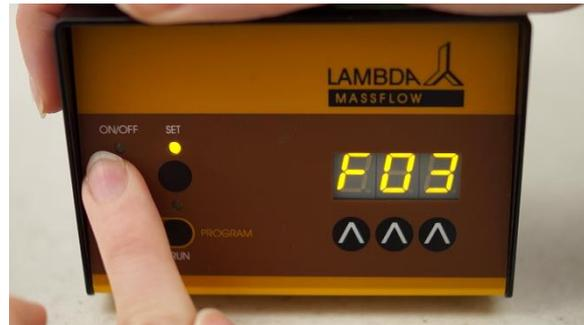
**Figure 2-10** After having entered the time of the last step, press the **ON/OFF** button. For example: **"F03"**
