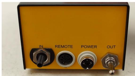
**Figure 1.1-2** Other end of the 8-pole cable should be connected to the REMOTE-socket at the rear of the MASSFLOW gas flow measurement and controller.
