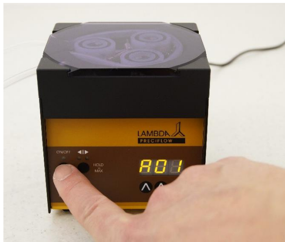
Figure 4-6 To confirm the address and save it, press the ON/OFF button.
