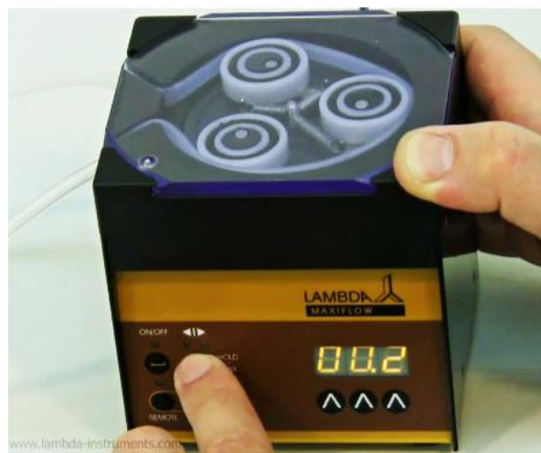
Figure 2-14 Press ◀▶ button, to set the time resolution.
